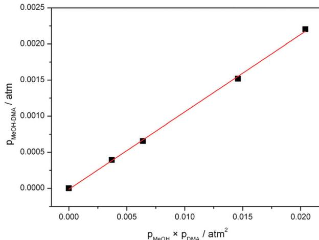
Fig. 5 Plot of  $p_{\text{MeOH–DMA}}$  against  $p_{\text{MeOH}} \times p_{\text{DMA}}$ .  $p_{\text{MeOH–DMA}}$  are determined from the experimental and theoretical fundamental OH-stretching transition intensities.
