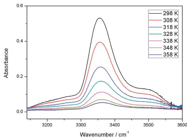
Fig. 7 The temperature dependence of the  $\tilde{\nu}_{\text{OH}}$  band in MeOH–TMA complex. A path length of 2.4 m was used. At a given temperature, the spectrum was obtained by subtracting the spectra of 32 Torr TMA and 22 Torr MeOH from the mixture of the two gases.
