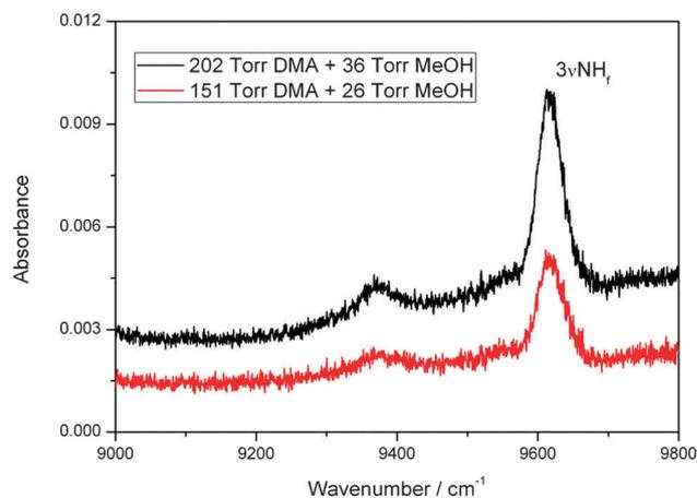
**Fig. 3** The  $3\tilde{\nu}_{\text{NH}}$  band of the MeOH–DMA complex obtained by spectral subtraction of  $202$  Torr DMA and  $36$  Torr MeOH from the mixture of the two gases (upper trace), and of  $151$  Torr DMA and  $26$  Torr MeOH from the mixture of the two gases (lower trace). The spectra were recorded in a  $4.8\text{ m}$  path length cell using an NIR light source and an InGaAs detector at  $297\text{ K}$ .
