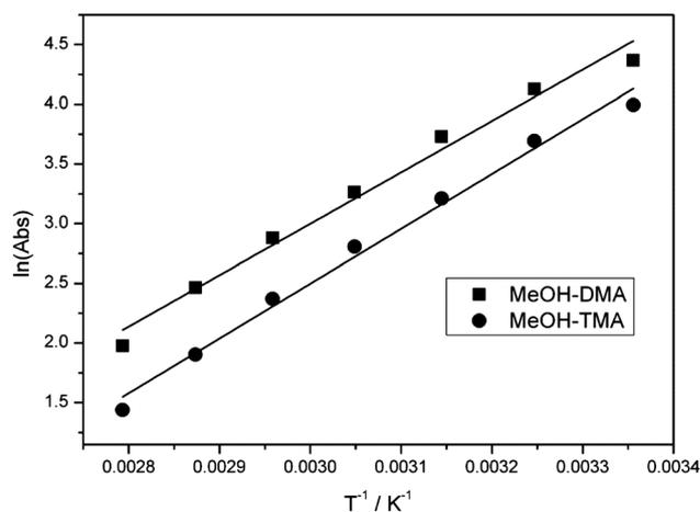
Fig. 8 The linear least-square fitting of the van't Hoff equation plot of the MeOH–DMA and MeOH–TMA complexes. Both bands were integrated in the  $\tilde{\nu}_{\text{OH}}$  band region between 3192 and 3580 cm<sup>-1</sup>.
