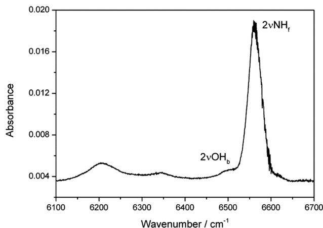
**Fig. 2** The  $2\tilde{\nu}_{\text{NH}_f}$  and  $2\tilde{\nu}_{\text{OH}_b}$  bands of the MeOH–DMA complex obtained by spectral subtraction of  $27$  Torr DMA and  $27$  Torr MeOH from the mixture of the two gases. The spectra were recorded in a  $4.8\text{ m}$  path length cell using an NIR light source and an InGaAs detector at  $297\text{ K}$ .
