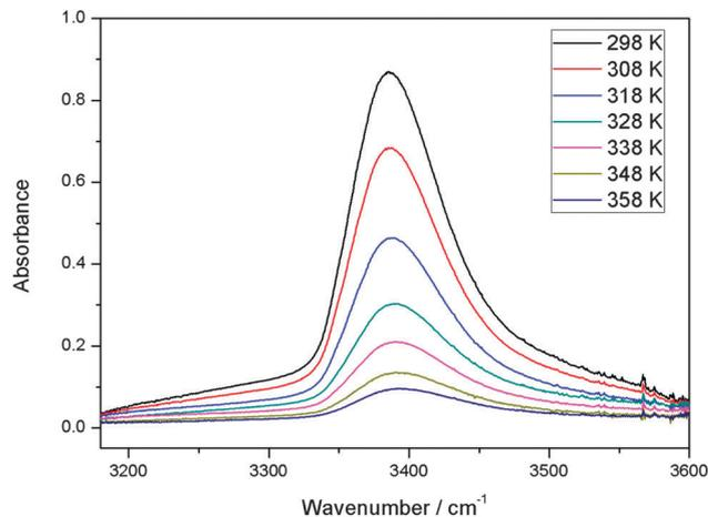
Fig. 6 The temperature dependence of the  $\tilde{\nu}_{\text{OH}}$  band in MeOH–DMA complex. A path length of 2.4 m was used. At a given temperature, the spectrum was obtained by subtracting the spectra of 64 Torr DMA and 22 Torr MeOH from the mixture of the two gases.
