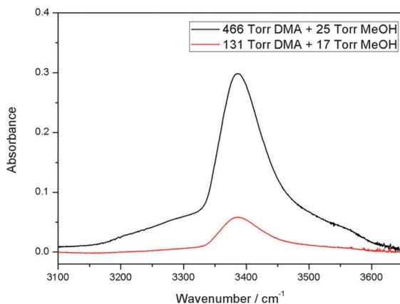
**Fig. 1** The  $\tilde{\nu}_{\text{OH}}$  transition of the MeOH–DMA complex obtained by spectral subtraction of 466 Torr DMA and 25 Torr MeOH from the mixture of the two gases (upper trace), and of 131 Torr DMA and 17 Torr MeOH from the mixture of the two gases (lower trace). All the spectra were recorded in a 10 cm path length cell using an MIR light source and an MCT detector at  $300 \pm 1$  K.
