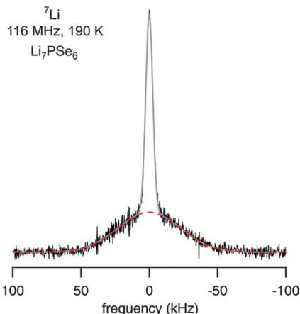
**Fig. 4**  $^7\text{Li}$  solid-echo (first-order quadrupolar) NMR spectrum recorded using a two-pulse sequence at 116 MHz and 190 K. The area fractions of the dipolar broadened central and quadrupole contribution are in agreement with the theoretical ratio of 4:6. Upon increasing temperature, the central line and the broad quadrupole signal narrow due to rapid Li exchange.
