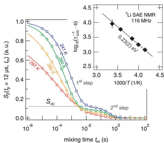
**Fig. 7**  $^7\text{Li}$  NMR (sin-sin) two-time correlation functions recorded using the Jeener-Broekaert<sup>38,39</sup> pulse sequence (116 MHz,  $t_p = 12 \mu\text{s}$ ). While the first decay step of the  $S_2$  decay curve reflects Li hopping between electrically inequivalent Li sites in crystalline  $\text{Li}_7\text{PSe}_6$ , the second one is induced by (quadrupolar) spin-lattice relaxation. Solid lines represent fits with a combination of two stretched exponentials.
