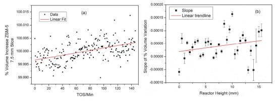
Fig. 5 (a) Volume change in ZSM-5 (expressed as a percentage of the average volume) for the 7.5 mm slice of the MTG reactor; (b) plot of slopes of the linear regression lines in the volume data for all slices of the reactor. Linear regression lines are shown to illustrate the trends in the data.
