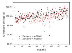
**Fig. 1** Percentage change in the volume of ZSM-5 for two different final refined values of the zero error correction in the parametric Rietveld refinement, during the MTG process in a slice of the reactor 3.5 mm from the inlet. TOS stands for "time on stream": the time for which the catalyst bed has been exposed to the methanol reagent gas. Refinement was carried out along the reactor slice (see Section B). Note the upward trend in the volume/average volume percentage.
