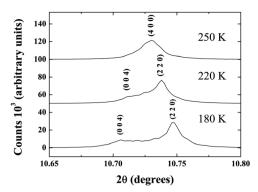
Fig. 2 A selected area of the synchrotron X-ray diffraction pattern of Ba<sub>2</sub>Gd-MoO<sub>6</sub> showing the [400] structural peak at 250 K (top). There is clear evidence of peak splitting at the cubic to tetragonal phase transition displayed here for T =220 K (middle) and 180 K (bottom). This peak splitting increases upon reducing the temperature.
