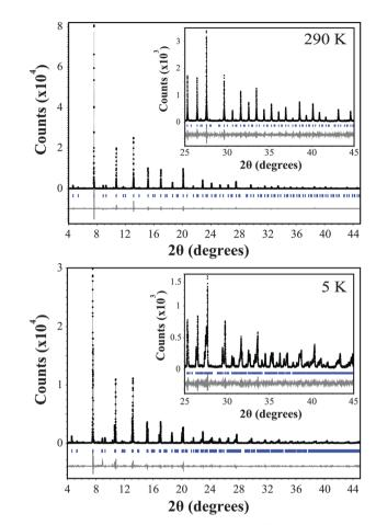
Fig. 1 Rietveld refinement of the synchrotron X-ray diffraction data for Ba<sub>2</sub>Gd-MoO<sub>6</sub>. The black line represents the actual data, the black circles represent the calculated pattern and the trace below is the difference between calculated and collected data. A region between 6.65 and 7.45  $2\theta$  (degrees) is excluded due to a peak associated with a small amount of unknown impurity.
