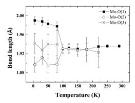
Fig. 5 The thermal evolution of the Mo–O bond lengths in  $Ba_2GdMoO_6$ . There is no evidence of the Jahn–Teller distortion previously reported for  $Ba_2LnMoO_6$  (Ln=Nd,Sm).
