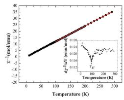
**Fig. 6** Inverse magnetic susceptibility data  $\chi^{-1}$  vs. T and  $d\chi^{-1}/dT$  vs. T (inset) for Ba<sub>2</sub>GdMoO<sub>6</sub>, evidencing the structural transition from tetragonal to triclinic symmetry below 100 K.
