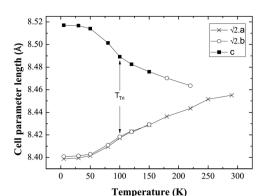
**Fig. 4** Evolution of the cell parameters with temperature evidencing a structural transition to triclinic symmetry below 100 K ( $T_{Tri}$ ); a and b have been multiplied by  $\sqrt{2}$  for ease of comparison.
