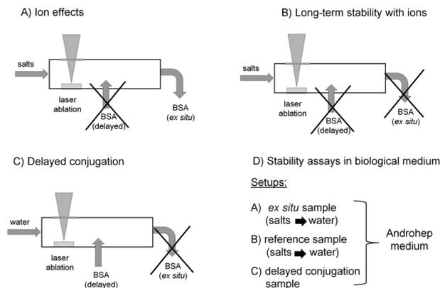
**Fig. 1** Experimental Au NP synthesis approaches for studying (A) ion effects, (B) long-term stability in the presence of ions, (C) delayed conjugation with BSA and (D) stability in Androhep biological medium.
