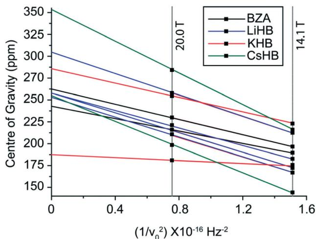
Fig. 8 The  $B_0$  variation of the centre-of-gravity shifts ( $\delta_{cg}$ ) measured from the  $^{17}\text{O}$  DOR data for BZA and the Group I alkali HD complexes.
