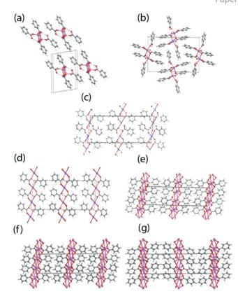
Fig. 3 The crystal packing schemes for the (a) LiHD, (b) NaDT, (c) KHD, (d) RbHD (6 coordinate monoclinic), (e) RbHD (8 coordinate monoclinic), (f) CsHD (monoclinic) and (a) CsHD (orthorhombic) systems
