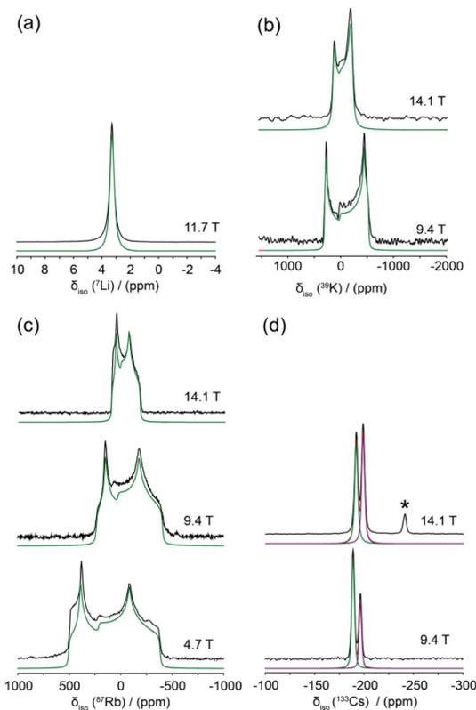
Fig. 9 The solid state NMR data of the Group I alkali metals, (a)  $^7\text{Li}$  MAS ( $\nu_r = 27.5$  kHz), (b) multiple field static  $^{39}\text{K}$ , (c) multiple field static  $^{87}\text{Rb}$  and (d) multiple field  $^{133}\text{Cs}$  MAS ( $\nu_r = 10$  kHz). The resultant simulations are shown below each spectrum in green and purple. The asterisk indicates the presence of Cs benzoate in this compound.
