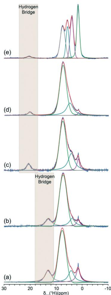
Fig. 4 Fast <sup>1</sup>H MAS NMR data ( $\nu_r = 27.5$  kHz,  $\nu_0 = 500.1$  MHz) acquired from (a) BZA, (b) LiHD, (c) KHD, (d) RbHD and (e) CsHD. The hydrogen bonded proton is marked in the shaded grey region.
