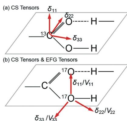
**Fig. 1** A schematic representation of the (a)  $^{13}\text{C}$  chemical shift (CS) tensor, and (b)  $^{17}\text{O}$  chemical shift and electric field gradient (EFG) tensors involved in carboxylic hydrogen bonded systems.
