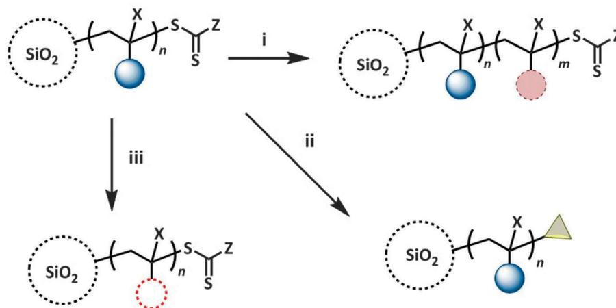
**Scheme 3** Post-polymerization modification of hybrid nanoparticles: (i) chain extension of RAFT-grafted polymer chain; (ii) modification of thiocarbonylthio end-group; (iii) modification of grafted polymer chain. X represents H or Me,  $n$  and  $m$  represent the number of monomer repeat units of the first and second block respectively.
