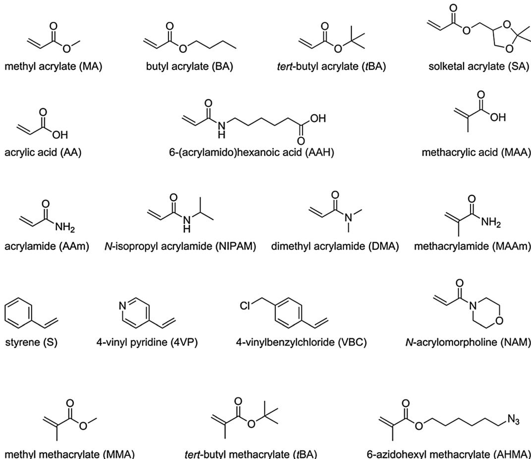
Fig. 2 Monomers grafted to silica surfaces using RAFT.
