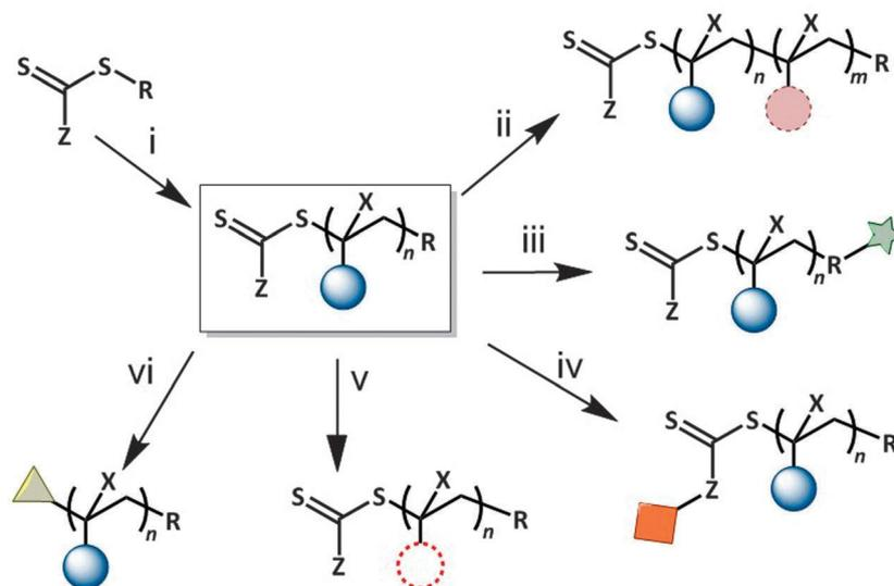
**Scheme 2** (i) RAFT polymerization of a vinyl-bearing monomer; (ii) chain-extension of the first block; (iii) modification of the R-group; (iv) modification of the Z-group; (v) modification of the polymer chain; (vi) modification of the thiocarbonylthio group. X represents H or Me,  $n$  and  $m$  represent the number of monomer repeat units of the first and second block respectively.
