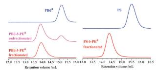
**Fig. 3** Syntheses of PBd-b-PE and PS-b-PE monitored by HT-SEC using TCB as an eluent at 150 °C. <sup>a</sup> The negative peak was shown with positive style for better comparison (dn/dc of PE and PBd are negative in TCB).
