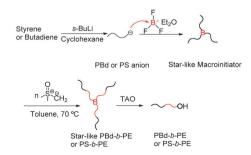
**Scheme 1** Combination of anionic polymerization and polyhomologation leading to PBd-b-PE and PS-b-PE block copolymers (BF<sub>3</sub>OEt<sub>2</sub>: "bridge" molecule).
