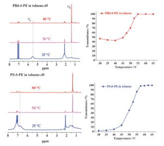
Fig. 6 Thermal responses of PBd-b-PE and PS-b-PE copolymers revealed by <sup>1</sup>H NMR in toluene-d<sub>8</sub> (left) at different temperatures and UCST measurements in toluene (3 mg mL<sup>-1</sup>) (right).
