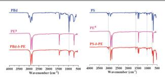
**Fig. 4** FTIR spectra of PBd-*b*-PE and PS-*b*-PE copolymers, <sup>a</sup>PE standard with a molecular weight of 2000.
