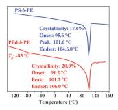
DSC curves of PBd-b-PE and PS-b-PE diblock copolymers.
