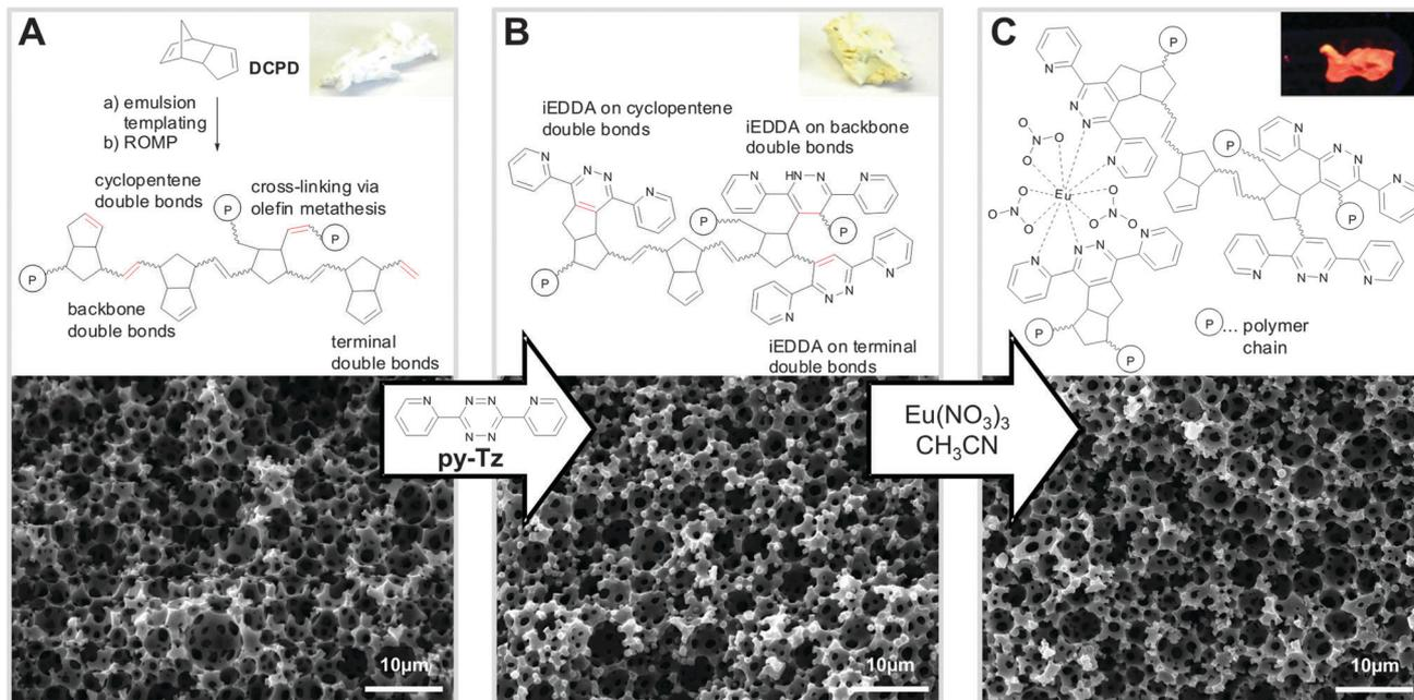
**Fig. 1** Representative chemical structures, SEM micrographs and photographs of (A) pDCPD foam, (B) after modification with 0.5 equiv. of **pyTz** (3,6-di(pyridin-2-yl)-1,2,4,5-tetrazine) and (C) after impregnation with  $\text{Eu}(\text{NO}_3)_3$  (photograph taken under UV light ( $\lambda = 365 \text{ nm}$ )).
