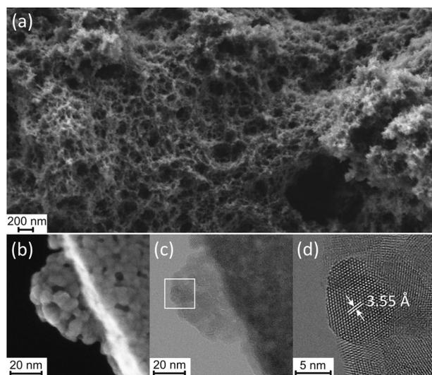
**Fig. 1** Images of the mesoporous solid **2**: (a) SEM image showing meso- and macropores; (b) STEM image showing nanosized pores; (c) the same fragment in TEM mode; (d) HRTEM image of a single particle showing the crystalline nature of the nanoparticle architecture (lattice fringes corresponding to the (102) reflections of trigonal  $\text{ZnCO}_3$ ).
