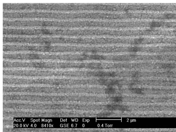
Fig. 2 SEM image of the surface of the DVD-RW Ag working electrode.
