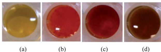
**Fig. 3** Small scale NQS colour testing with addition of heat performed in plastic micro-well plates on a blank control reagent (a), BZP HCl (b), ephedrine HCl (c), and 4-MMC HCl (d) sample solutions.
