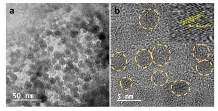
Fig. 2 (a) TEM image of Zn-Cdots (50 nm scale bar). (b) HRTEM image showing Zn-Cdots with an average size  $4.8 \pm 0.8$  nm (5 nm scale bar).
