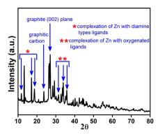
Fig. 3 The PXRD spectrum of Zn-Cdots.
