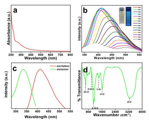
Fig. 1 (a) UV-Vis spectrum of Zn-Cdots dispersed in water at a concentration of 0.25 mg mL<sup>-1</sup>. (b) Excitation-dependent emission of Zn-Cdots dispersed in water at 0.5 mg mL<sup>-1</sup> concentration (inset: images of aqueous solution of Zn-Cdots under daylight and UV light). (c) Excitation (wavelength 330 nm) spectrum of Zn-Cdots corresponding to the 411 nm emission peak. (d) FTIR spectrum of Zn-Cdots
