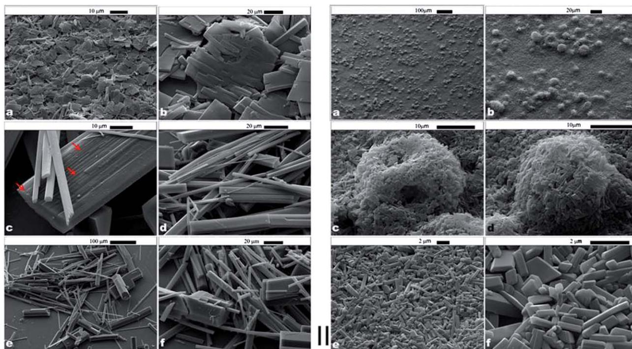
**Fig. 3** (I)  $\alpha$ -CD-tetradecane ICs: (a) and (b) lamella plate structures; (c) lamella sheets formed from stacking of long microrods shown by red arrows; (d) long microrods responsible for forming lamella plates; (e) and (f) some IC microrods showing different cross-sectional areas. (II)  $\beta$ -CD-tetradecane ICs: (a) to (d) spherical structures formed by heating up of  $\beta$ -CD-tetradecane ICs. (e) and (f) Short microrods formed  $\beta$ -CD-tetradecane ICs.
