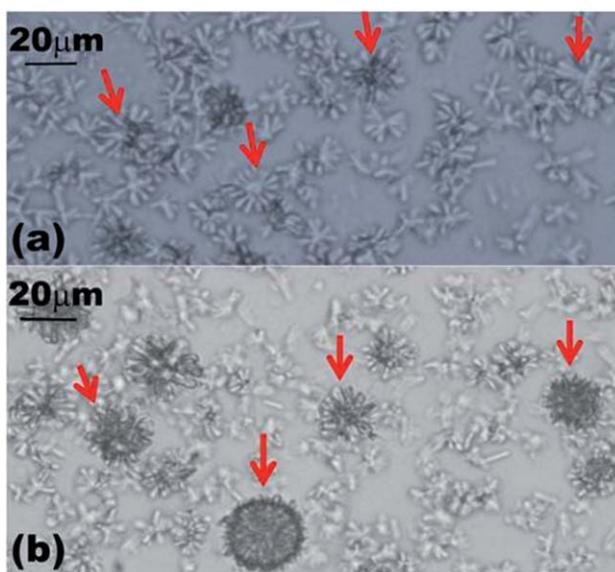
**Fig. 6** Optical images showing the formation of spherical structures by  $\alpha$ -CD-tetradecane ICs after dissolving the microrods by heating them at 85  $^{\circ}$ C before cooling to room temperature. (a) Optical micrographs showing the process of forming spherical structures 5 minutes after the aqueous solution was deposited on the microscope glass slide from a hot bath. (b) The same sample 15 minutes later on the microscope slide.
