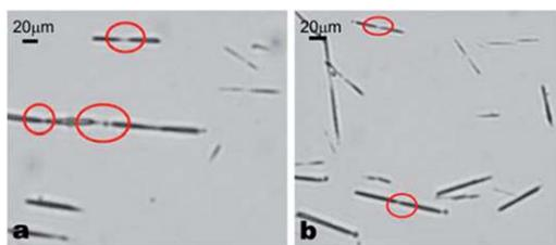
**Fig. 11**  $\alpha$ -CD–tetradecane ICs prepared in 1 M urea solution showing some end-to-end joining which leads to their elongation with time. The end-to-end connections are highlighted by red circles.
