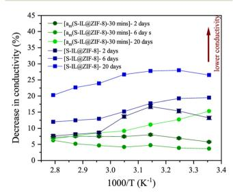
Fig. 10 Change in the ionic conductivity of crystalline (square) and amorphous composite (circle). Reproduced from open access journal
