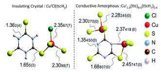
Fig. 5 Local structure and bond lengths of Cu<sup>I</sup>Cl(ttcH<sub>3</sub>) and Cu<sup>I</sup><sub>1.8</sub>(ttc)<sub>0.6</sub>(ttcH<sub>3</sub>)<sub>0.4</sub>. Reproduced from ref. 15 with permission from Royal Society of Chemistry, copyright 2015.
