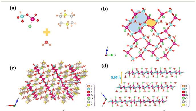
Fig. 1 (a) The  $[Zn(H_2PO_3)Cl_2]^-$  unit,  $(C_4H_{12}N_2)^{2+}$  cation and crystalline water molecules; (b) the  $\{[Zn_2Cl_2(HPO_3)_2(H_2O)_2]_{\infty}\}^{2-}$  layer in the bc plane; (c) overall crystal structure viewed along the b direction; (d) the arrangement of the  $\{[Zn_2Cl_2(HPO_3)_2(H_2O)_2]_{\infty}\}^{2-}$  layers along the b-axis.
