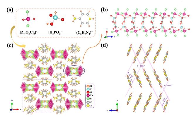
Fig. 2 The crystal structure of  $(C_5H_7N_2)[Zn(H_2PO_3)Cl_2]$ . (a) The  $[ZnO_2Cl_2]^{4-}$ , the  $[H_2PO_3]^-$  unit, and the  $\pi$ -conjugated  $(C_5H_7N_2)^+$  group; (b) the  $\{[Zn(H_2PO_3)Cl_2]_\infty\}^-$  chains; (c) the whole crystal structure viewed from the c axis; (d) the  $\pi$ -conjugated  $(C_5H_7N_2)^+$  groups viewed along the b axis and the dihedral angle between two alternating orientations.
