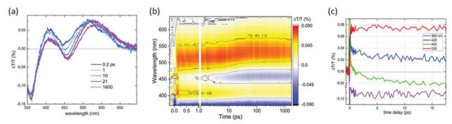
Fig. 3  $\Delta T/T$  spectra of C-dots produced by the space-confined vacuum-heating approach: (a) spectra for selected time delays, (b) map, (c) dynamics for selected wavelengths; pump@400 nm with fluence of 6.5 mJ cm<sup>-2</sup>, pump and probe polarization are set at magic angle.
