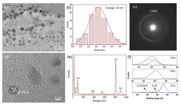
Fig. 1 Typical TEM image (a) and size distribution (b) of the C-dots synthesized *via* the vacuum heating approach. (c) SAED pattern and (d) HRTEM image of the C-dots. (e) EDS of the C-dots. (f) High-resolution XPS spectra of the C-dots.
