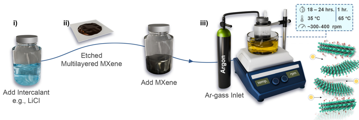
Scheme 4 (i) Depiction of LiCl addition to DI water. (ii) Mixing of the ml-MXene cake with LiCl solution. (iii) Laboratory setup and processing conditions.
