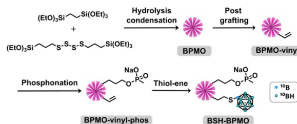
Fig. 2 BSH-BPMO synthetic pathway.
