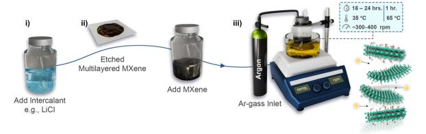
Scheme 4 (i) Depiction of LiCl addition to DI water. (ii) Mixing of the ml-MXene cake with LiCl solution. (iii) Laboratory setup and processing conditions.
