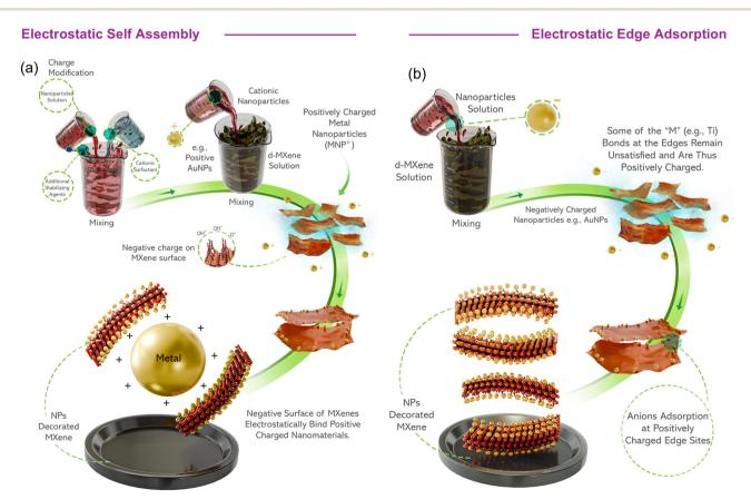
Fig. 4 Schematic demonstration of the (a) possible pathway for charge inversion and electrostatic self-assembly with negatively charged MXene. (b) Electrostatic adsorption of negatively charged nanoparticles with positive edges of MXene flakes.
