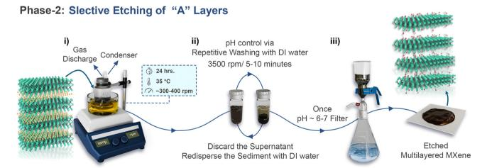
Scheme 3 (i) Laboratory settings typically followed for etching (ii) washing procedure for pH control. (iii) Depiction of the filtration assembly and asetched MXene cake obtained after filtration. Note: this method is universal for almost all MAX phases etched via the wet-chemical route.
