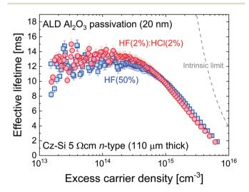
Fig. 6 Effective lifetime versus excess carrier density for 110 µm thick 5  $\Omega$  cm n-type Cz-Si samples from the same wafer treated with HF (2%): HCl(2%) or HF(50%) for 10 min immediately before the ALD process (200 °C deposition with 460 °C activation). The level of surface passivation is the same within the 5% error shown, unlike for the superacid-derived passivation in Fig. 1(b). The intrinsic lifetime limit from Richter et al. 23 is also shown.
