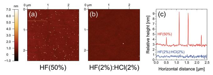
Fig. 5 Representative 25  $\mu$ m  $\times$  25  $\mu$ m AFM maps of 5  $\Omega$  cm n-type FZ-Si after (a) an HF(50%) treatment for 10 min and (b) an HF(2%): HCl(2%) treatment for 10 min. Neither sample had been subsequently treated with superacid-derived passivation. The horizontal line scans in (c) show scans typical of both sample types.
