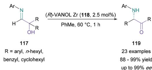
**Scheme 25** Wulff's (*R*)-VANOL Zr-catalysed enantioselective iminol rearrangement.
