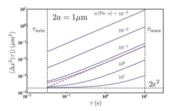
**Fig. 3** Calculated mean-squared displacements for 1  $\mu$ m diameter probe particles in fluids of increasing viscosity from  $10^{-3}$  to 10 Pa·s. The operating regime for multiple particle tracking microrheology is defined by the shortest and longest lag times and the particle tracking error. Solid curves are the apparent MSD, while the dashed line for  $\eta = 0.146$  Pa s is the true MSD.
