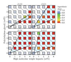
**Fig. 5** Gelation state diagram for a PEG ( $M_n$  5 000)-HMWH hydrogel. The logarithmic slope of the MSD is  $\alpha = d \log \langle \Delta r^2(\tau) \rangle / d \log \tau$ . Reprinted with permission from K. M. Schultz, A. D. Baldwin, K. L. Kiick and E. M. Furst, *Macromolecules*, 2009, **42**, 5310–5316. Copyright 2009 American Chemical Society.
