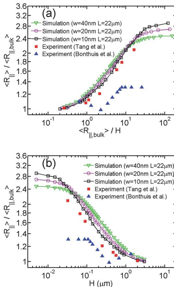
**Fig. 7** (a) Relative in-plane radius of gyration as a function of the inverse relative slit height. Three lines with open symbols correspond to the simulations #8, #9 and #10 in Table 1. Red squares are the data of Tang *et al.*<sup>26</sup> Blue triangles are the data of Bonthuis *et al.*<sup>25</sup> (b) Relative in-plane radius of gyration as a function of the slit height.
