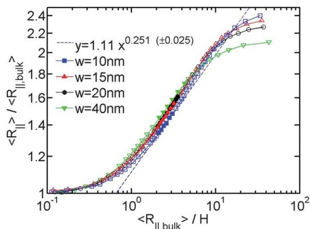
**Fig. 3** Relative in-plane radius of gyration as a function of the inverse of relative slit height for the simulation #5,#6,#7,#2 in Table 1. The filled symbols are the data points in both extended de Gennes and de Gennes regimes. The open symbols are the data points in other regimes. The blue dashed line is a best power law fit to the filled blue squares. ( $\pm 0.025$ ) refers to the uncertainty of the exponent from the fits. The uncertainty for the prefactor is  $1.11 \pm 0.03$ .
