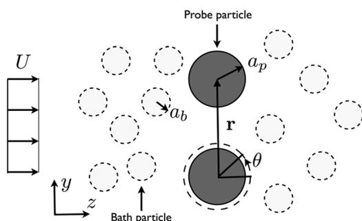
**Fig. 1** Experimental configuration. Two probes are held using a time shared optical trap. The probe particle and bath particle have radii of  $a_p$  and  $a_b$ , respectively. The velocity of the flow is indicated by  $U$ . The center-to-center distance between the probes is indicated by  $r$ .
