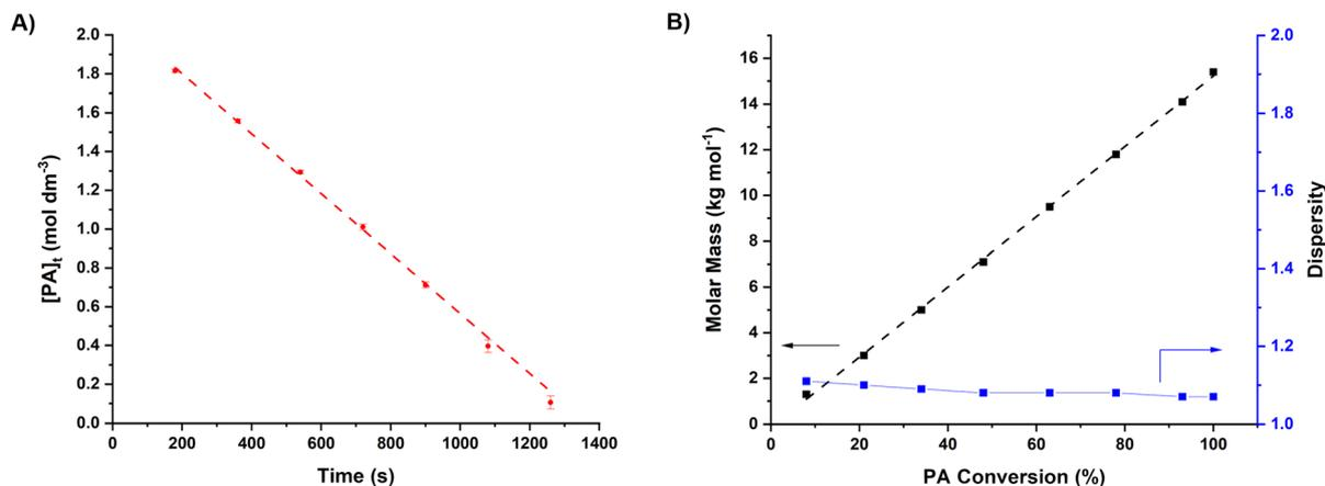
**Fig. 2** Catalyst benchmark data for the ROCOP of CHO and PA with complex 2. Conditions: [2] : [PA] : [CHO] = 1 : 400 : 2000,  $T = 100\text{ }^{\circ}\text{C}$ . (A) Plot of  $[\text{PA}]_t$  vs. time (s). Reaction displays a zero-order dependence on  $[\text{PA}]_t$ . Reactions repeated in triplicate, with average values of  $[\text{PA}]_t$  plotted. (B) Plot of polymer molar mass, and dispersity, against PA conversion.
