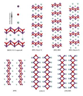
Fig. 1 Slab models for {010}, {110} and {001} surfaces of BiOX.
