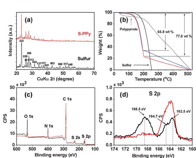
**Fig. 2** (a) XRD patterns of sulfur (black) and the S-PPy composite (red), (b) thermogravimetric analysis (TGA) of sulfur (black), pristine PPY (grey), and S-PPy composites (red and blue), showing up to 77 wt% of sulfur contained within the composites, (c) XPS of S-PPy composite before (black) and after (red) sputtering, and (d) S 2p characteristic peaks in the XPS of S-PPy composite before (black) and after (red) sputtering.
