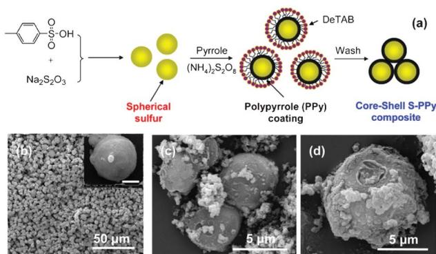
**Fig. 1** (a) Schematic illustration of the synthesis process of core-shell structured sulfur-polypyrrole (S-PPy) composites with the use of the cationic surfactant decyltrimethylammonium bromide (DeTAB), (b) scanning electron microscopy (SEM) image of the spherical sulfur particles with the inset showing a magnified SEM image of a single sulfur particle with a scale bar of 5  $\mu\text{m}$ , (c) SEM image of a few S-PPy composite particles, and (d) SEM image of a single S-PPy particle.
