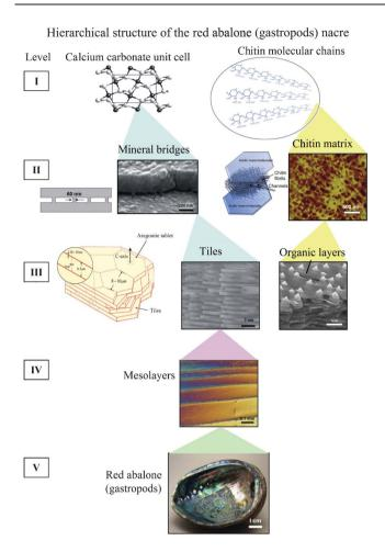
Fig. 3 Hierarchical structure (5 levels) of the red abalone (gastropod) nacre from nano, to micro, to meso, to structural length scales.<sup>26</sup>
