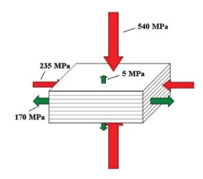
Fig. 13 Compressive and ultimate tensile strengths of nacre under different loading directions.<sup>32</sup>
