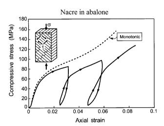
**Fig. 15** Compression stress–strain curves for nacre in abalone, representing interlamellar shear, measured both in monotonic loading and with loading–unloading loops. The insert indicates that the lamellae boundaries are orientated at 45° to the loading axis.<sup>5</sup>
