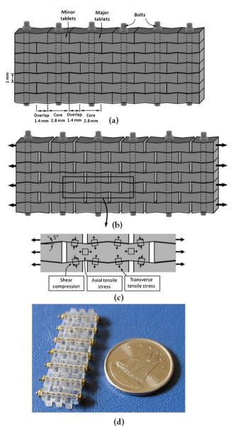
**Fig. 20** Overview of the nacre-like composites: (a) schematic with dimensions; (b) tablets under tension slide with progressive locking; (c) some of the stresses involved in progressive locking; (d) actual composite after assembly.<sup>1</sup>
