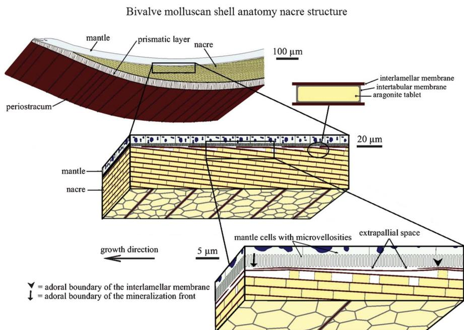
**Fig. 1** Schematic of the bivalve molluscan shell anatomy. It is composed of periostracum, a prismatic layer and nacre. The liquid-filled interlamellar space exists between the mineralized shell and the mantle part of the soft body of the organism. The schematic also illustrates successive amplifications of the brick and mortar structure of nacre. The growth surface, on which the patterns are observed, is between the mantle and the shell, and extends into the page.<sup>3</sup>
