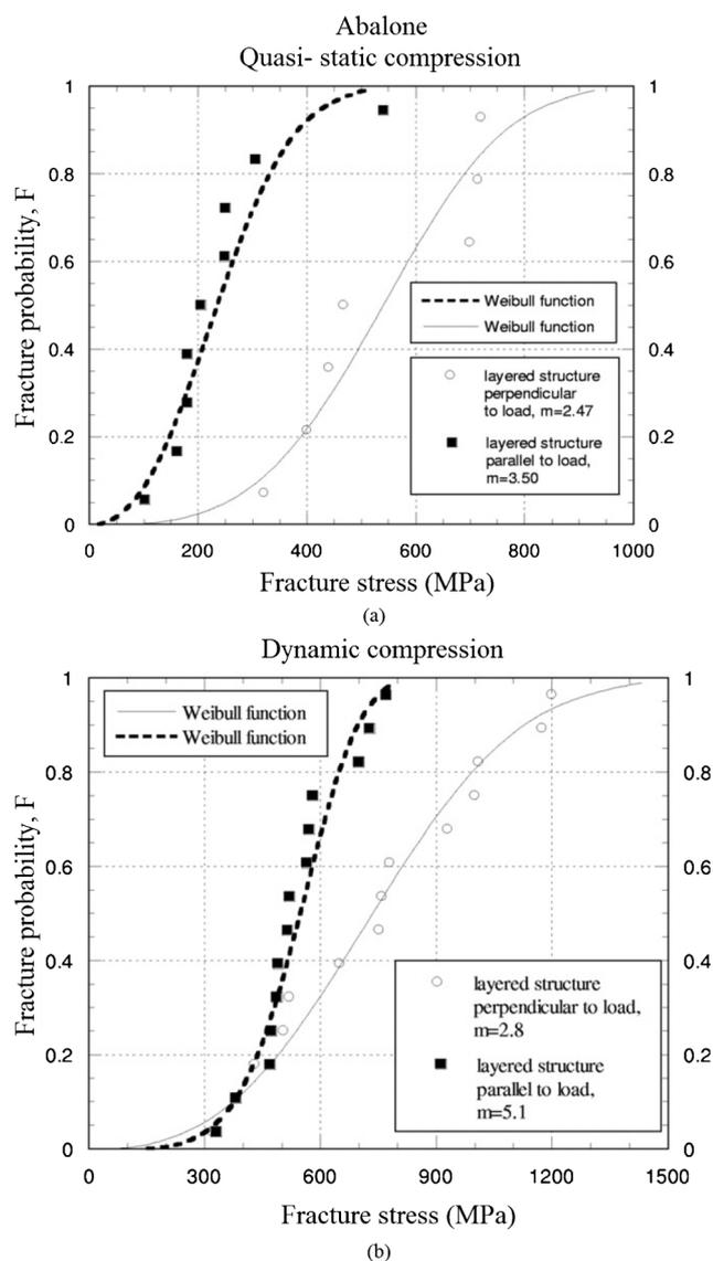
**Fig. 16** Weibull plots of abalone nacre in abalone under (a) quasi-static, and (b) dynamic compressive loading.<sup>46</sup>
