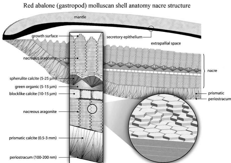
**Fig. 2** Schematic of the red abalone (gastropod) molluscan shell anatomy, showing a vertical section of the outer edge of the shell and mantle with an enlargement indicating the thickness dimensions of the shell structures. The size of the extrapallial space is exaggerated for clarity.<sup>2,112</sup>
