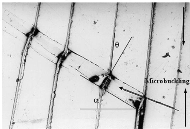
**Fig. 9** Mechanisms of damage accumulation in the nacreous region of abalone through plastic microbuckling.<sup>46</sup>
