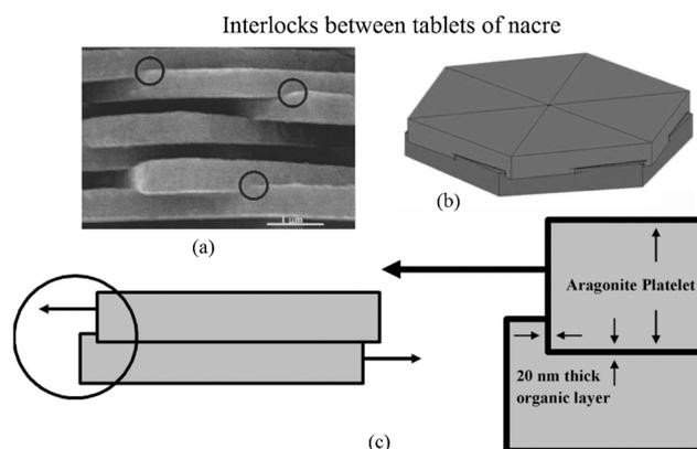
**Fig. 11** (a) SEM image of nacre from red abalone showing the presence of interlocks, indicated by circles; (b) schematic illustration showing interlocks between platelets of nacre, showing that rotation of layers of platelets is essential for the formation of platelet interlocks. (c) Schematic illustration showing the mechanism of loading through a cross-section cut across platelets and through the interlocks.<sup>41</sup>
