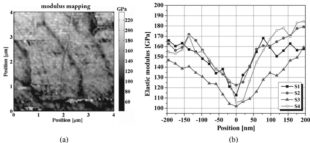
**Fig. 18** (a) Map of elastic modulus taken from the nacre layer at a depth of 300  $\mu\text{m}$  beneath the inner surface of the bivalve shells of *Perna canaliculus*; (b) the modulus change across organic–inorganic interfaces.<sup>110</sup>
