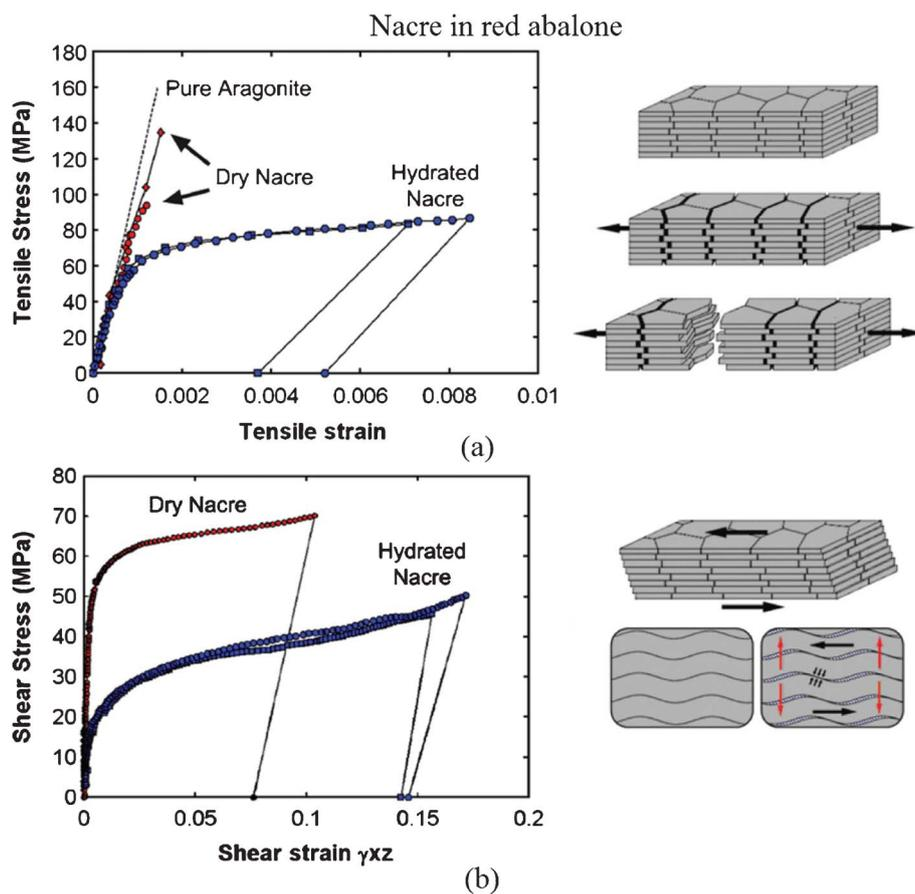
**Fig. 14** (a) Tensile and (b) shear stress–strain curves for nacre in red abalone and a schematic of lamellar tile structures showing associated deformation modes. Tablet waviness generates resistance to sliding, accompanied by lateral expansion (vertical arrows).<sup>48,104</sup>
