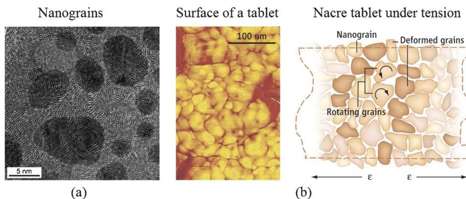
**Fig. 8** (a) High-resolution TEM (face-on view) of a tablet from the nacreous layer of a red abalone specimen showing nanograins of about 3–10 nm in size;<sup>31</sup> (b) (left) AFM image of surface nanograins on an individual nacre platelet from California red abalone and (right) schematic of nanograin rotation under tension.<sup>38,39</sup>
