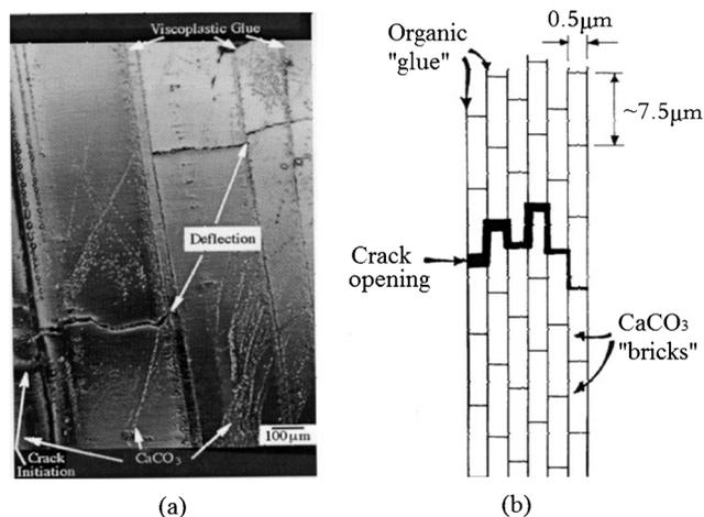
**Fig. 10** (a) Cross-section of abalone shell showing how a crack, starting at the left, is deflected by the viscoplastic layer between calcium carbonate lamellae; (b) schematic drawing showing the arrangement of calcium carbonate in nacre, forming a miniature “brick and mortar” structure.<sup>97</sup>
