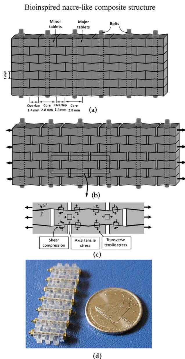
**Fig. 20** Overview of the nacre-like composites: (a) schematic with dimensions; (b) tablets under tension slide with progressive locking; (c) some of the stresses involved in progressive locking; (d) actual composite after assembly.<sup>1</sup>
