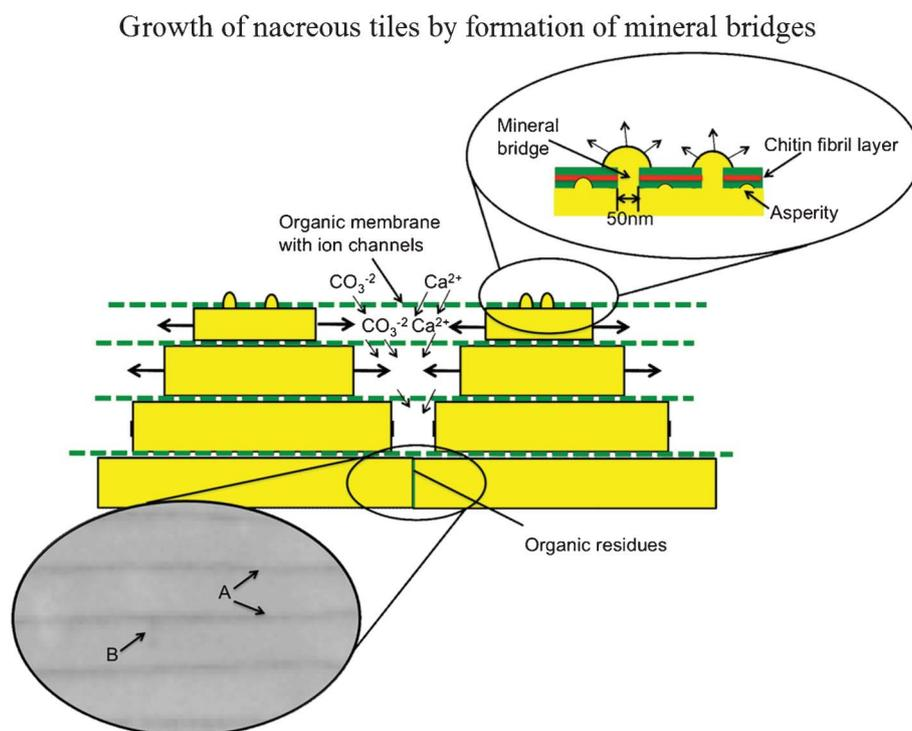
**Fig. 6** Mechanism of growth of nacreous tiles in abalone by formation of mineral bridges; the organic layer is permeable to calcium and carbonate ions, which nourish lateral growth as periodic secretion and deposition of the organic intertile membranes restricts their flux to the lateral growth surfaces. Arrows A designate the organic interlayer imaged by SEM; arrow B designates the lateral boundary of the tile.<sup>86</sup>
