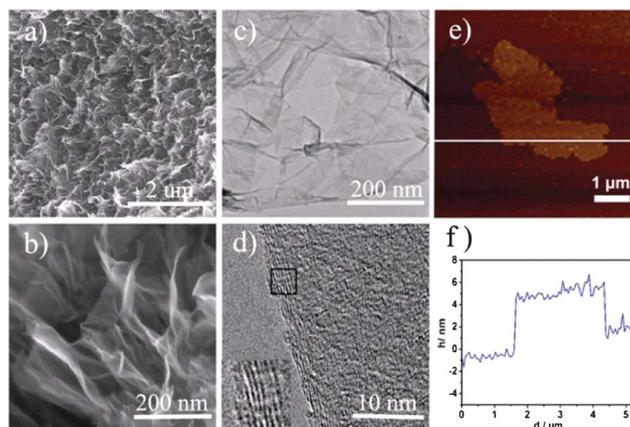
**Fig. 1** a, b) SEM, c) TEM and d) HR-TEM images of the NGS-1 (mass ratio of urea/GO is 300 : 1, 180  $^{\circ}$ C, 12 h); e) Representative AFM image and f) corresponding thickness analysis taken around the white line in e) reveal a thickness of 4–4.5 nm for NGS-1.
