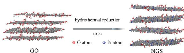
**Scheme 1** Schematic procedure for preparation of NGS.
