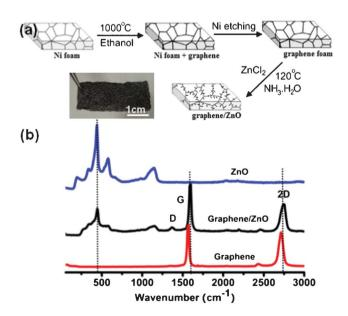
Fig. 1 (a) Schematic of the synthesis process and a photograph of graphene/ZnO hybrid. (b) Raman spectra of bare 3D graphene, ZnO and graphene/ZnO hybrid.
