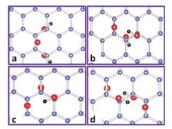
**Fig. 5** Some representative basic building blocks of GO with both epoxy and hydroxyl functional groups. Carbon, oxygen, and hydrogen atoms are indicated by blue, red, and black balls, respectively. (a) and (b): O + 2OH. (c): 2O + OH. (d): 2O + 2OH. Reprinted with permission from ref. 103 as follows: J. A. Yan *et al.*, *Physical Review B*, 2010, **82**, 125403. Copyright (2010) by the American Physical Society.
