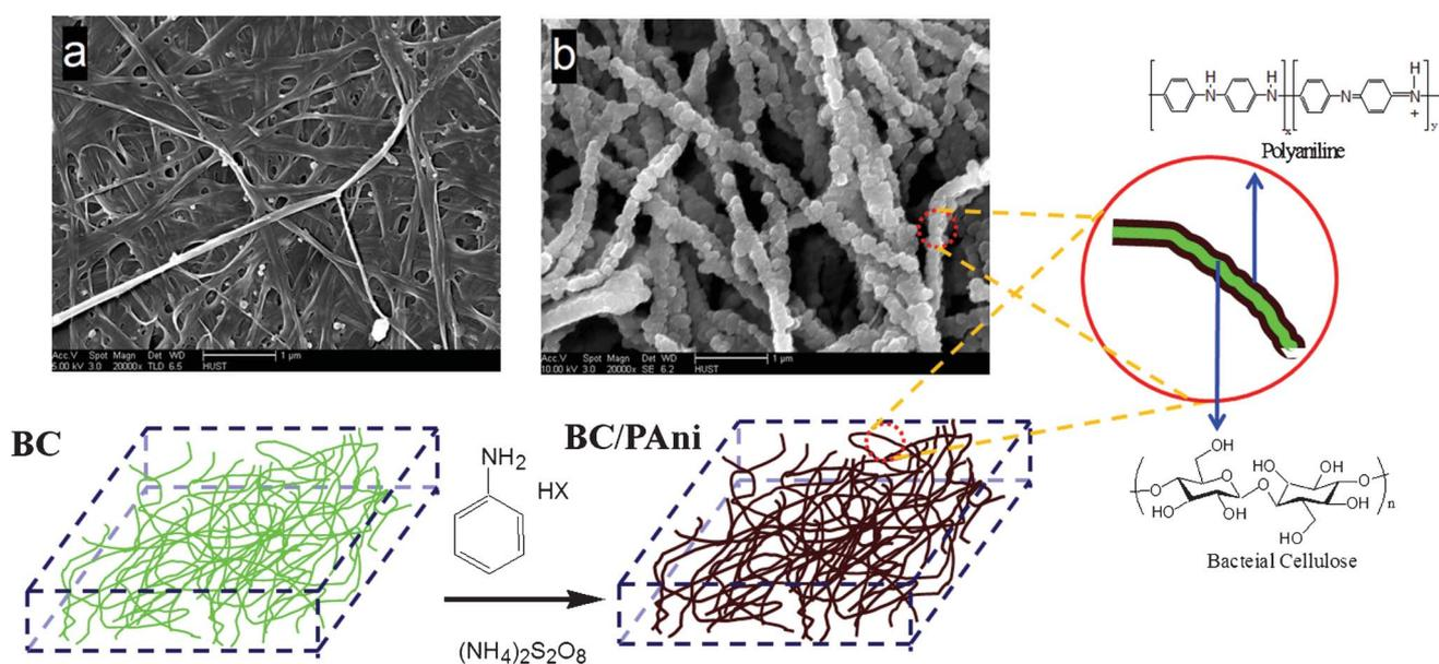
**Fig. 4** Schematic diagram of the process of aniline polymerization in the BC hydrogel. (Fig. a is the FESEM image of the hot-pressed BC membrane; and Fig. b is the FESEM image of hot-pressed BC-PAni membrane.)
