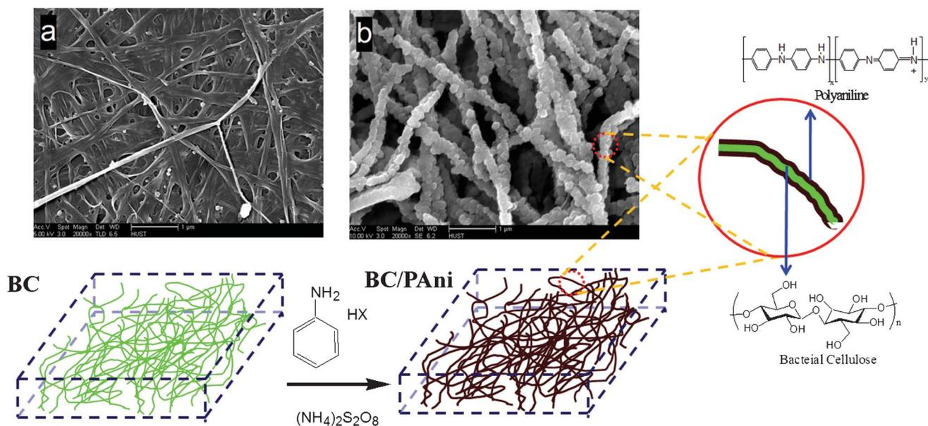
**Fig. 4** Schematic diagram of the process of aniline polymerization in the BC hydrogel. (Fig. a is the FESEM image of the hot-pressed BC membrane; and Fig. b is the FESEM image of hot-pressed BC-PAni membrane.)
