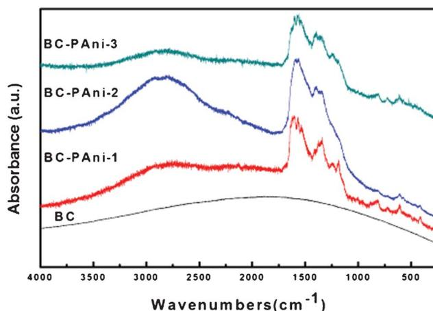
Fig. 9 Laser Raman spectra of BC and BC-PANI.
