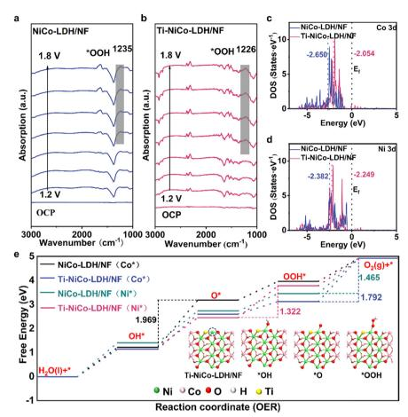
Fig. 4 In situ spectroscopic characterization: (a) NiCo-LDH/NF; (b) Ti-NiCo-LDH/NF; (c and d) the calculated DOS of NiCo-LDH/NF and Ti-NiCo-LDH/NF; (e) the OER free energy diagram for AEM steps and optimized intermediate geometry for Ni sites of Ti-NiCo-LDH/NF (inset).
