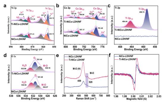
Fig. 2 Chemical states and electronic structural characterization of NiCo-LDH/NF and Ti-NiCo-LDH/NF. High-resolution XPS spectra of (a) Ni 2p, (b) Co 2p, (c) Ti 3d, and (d) O 1s; (e) Raman spectra; (f) EPR spectra.
