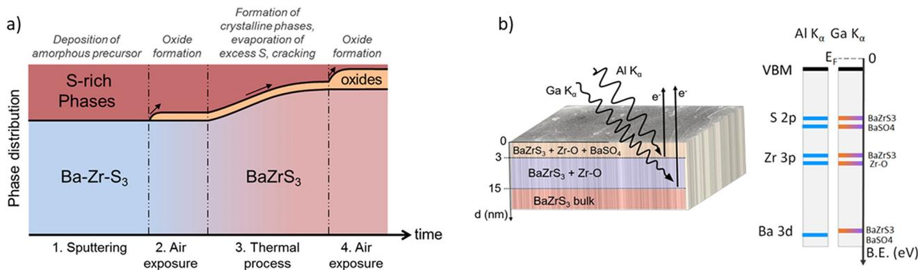
**Fig. 17** Surface oxide impurities in BaZrS<sub>3</sub>. (a) Schematic representation of phase distribution in the BaZrS<sub>3</sub> film over time upon exposure to air. (a) Reproduced with permission.<sup>97</sup> Copyright 2020, American Chemical Society. (b) Schematic illustrating the different phases present in the near-surface layers, as identified by hard X-ray photoelectron spectroscopy. (b) Reproduced with permission.<sup>139</sup> Copyright 2024, American Chemical Society.
