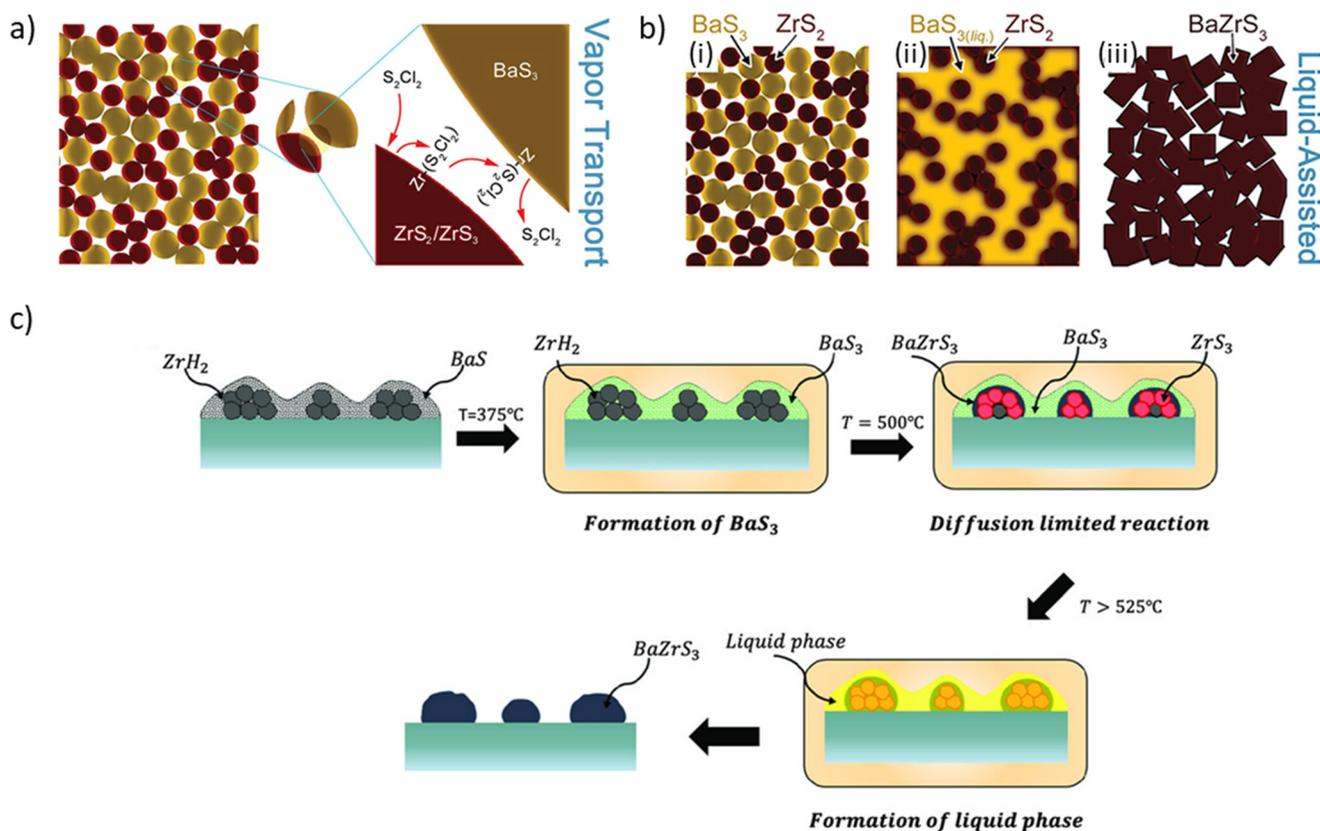
**Fig. 10** Schematic illustrating the working principles of: (a) S<sub>2</sub>Cl<sub>2</sub> vapor transport agent, (b) BaS<sub>3</sub> liquid flux, and (c) BaS<sub>x</sub> (x > 3) liquid flux. (a) Reproduced with permission.<sup>100</sup> Copyright 2023, American Chemical Society. (b) Reproduced with permission.<sup>101</sup> Copyright 2023, Wiley.
