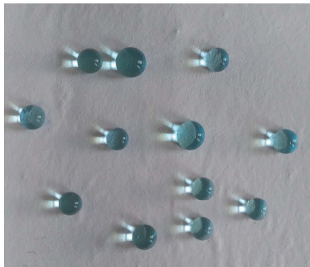
Fig. 6 Photograph of water droplets (dyed with methylene blue) on the M-4 surface.
