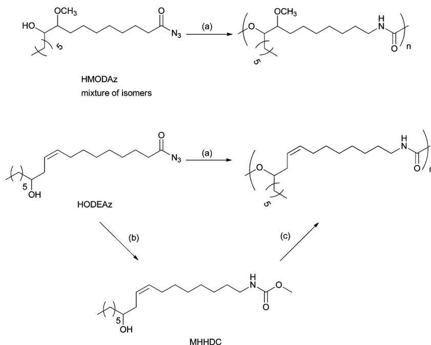
**Scheme 9** Polyurethane prepared from functionalized oleic acid and ricinoleic acid (a) 80 °C, 24 h (for clarity only the 10-hydroxy-9-methoxy isomer of HMODAz is presented); (b) CH<sub>3</sub>OH, reflux, 4 h; (c) Ti(OBu)<sub>4</sub>, 130 °C, 6 h.
