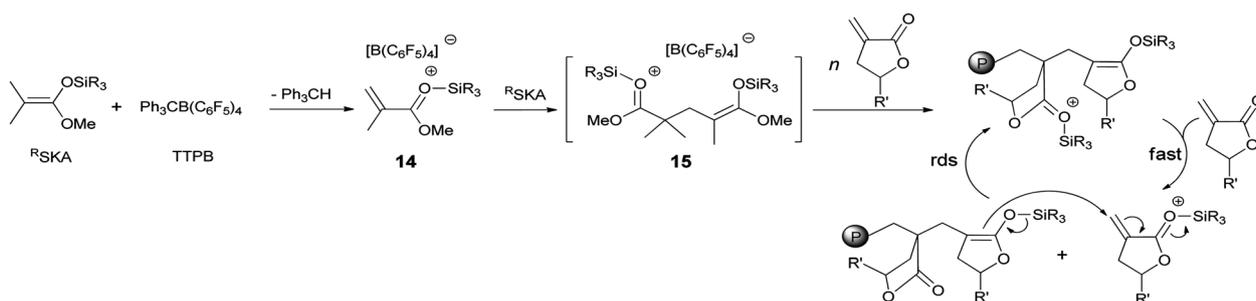
**Scheme 4** Proposed mechanism for the polymerization of (M)MBL with ambiphilic silicon propagators ( $R' = \text{H}$  or  $\text{CH}_3$ ).
