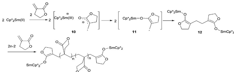
**Scheme 3** Proposed mechanism for the polymerization of MBL with Cp\*<sub>2</sub>Sm(THF)<sub>2</sub>.
