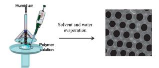
**Fig. 1** Basic "breath figures" casting technique for the formation of honeycomb structured porous polymer membranes (left). Microscopy image of a typical honeycomb structured porous film (right).
