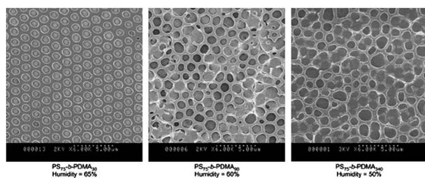
**Fig. 6** SEM images of films cast from PS-*b*-PDMS ( $10 \text{ g L}^{-1}$  in  $\text{CS}_2/\text{CH}_2\text{Cl}_2$  70 : 30 v/v%) showing that the regularity is compromised with increasing length of the hydrophilic PDMA block. Re-printed from K. H. Wong, T. P. Davis, C. Barner-Kowollik and M. H. Stenzel, Honeycomb structured porous films from amphiphilic block copolymers prepared via RAFT polymerization, *Polymer*, 2007, **48**, 4950–4965.
