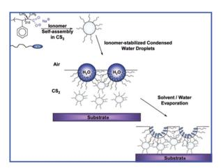
**Fig. 11** Representation of the formation of the honeycomb structured films by ionomer-stabilized condensed water droplets. The pores possess a functionality. Re-printed from L. Billon, M. Manguian, V. Pellerin, M. Joubert, O. Eterradossi and H. Garay, Tailoring highly ordered honeycomb films based on ionomer macromolecules by the bottom-up approach, *Marcromolecules*, 2009, **42**, 345–356.
