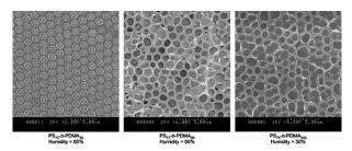
**Fig. 6** SEM images of films cast from PS-*b*-PDMS (10 g  $L^{-1}$  in CS<sub>2</sub>/CH<sub>2</sub>Cl<sub>2</sub> 70: 30 v/v%) showing that the regularity is compromised with increasing length of the hydrophilic PDMA block. Re-printed from K. H. Wong, T. P. Davis, C. Barner-Kowollik and M. H. Stenzel, Honeycomb structured porous films from amphiphilic block copolymers prepared *via* RAFT polymerization, *Polymer*, 2007, **48**, 4950–4965.
