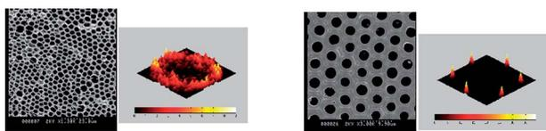
**Fig. 9** Honeycomb structured porous films and 3D contour plots from the QVLS analysis showing a halo geometry (left) indicating some repeated distances but not repeated angles and 6 peaks (right) resulting from the ideal hexagonal array in the film. Reprinted from S. D. Angus and T. P. Davis, *Polymer surface design and infomatics: facile microscopy/image analysis techniques for self-organizing microporous polymer film characterization*, *Langmuir*, 2002, **18**, 9547–9553.
