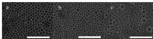
**Fig. 5** SEM images of the honeycomb structure of films prepared at 18 °C and 90% RH by spreading 40 μL of the copolymer solution (0.75 mg mL<sup>-1</sup>) onto (a) mica, (b) glass, and (c) silicon plates, respectively. The bar is 20 μm. Re-printed from C. Xia Cheng, Y. Tian, Y. Qiao Shi, R. Pei Tang and F. Xi, Porous polymer films and honeycomb structures based on amphiphilic dendronized block copolymers, *Langmuir*, 2005, **21**, 6576–6581.
