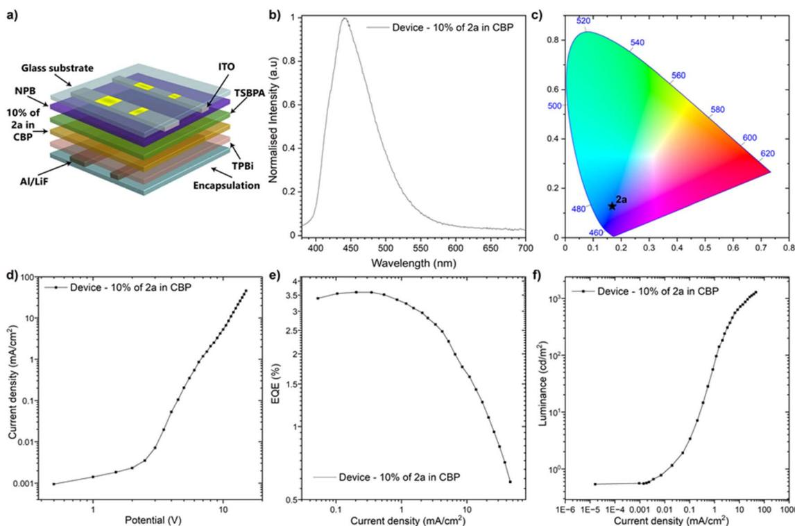
Fig. 5 OLED device characteristic: (a) schematic of an OLED device structure with a **2a** active layer, (b) electroluminescence spectrum of the studied device, (c) CIE 1931 chromaticity diagram indicating blue emission, (d) current density – potential, (e) external quantum efficiency–current density and (f) luminance–current density characteristics of the studied device.
