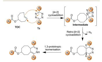
Scheme 3 The proposed mechanism of the IEDDA reaction.
