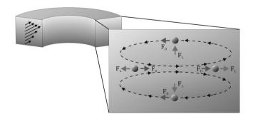
**Fig. 1** Schematic illustration of a continuous curved rectangular microchannel in which both the Dean force  $(F_{\rm D})$  and lift force  $(F_{\rm L})$  are present as well as the directions of their applied force on the particles, resulting in a single equilibrium position at the inner wall of the microchannel, where both forces operate in opposite directions.
