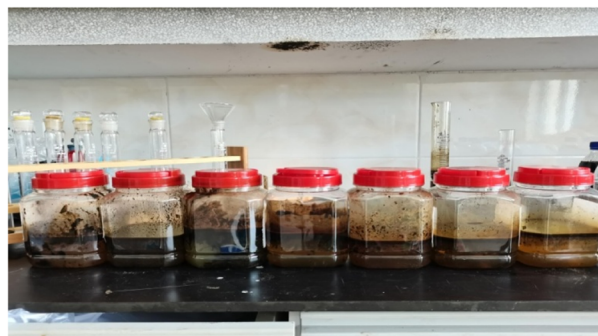
Fig. 7 Photographs of sludge and oil–water mixtures produced after pyrolysis. (a) Photograph of oily sludge samples after pyrolysis. (b) Photograph of oil–water mixtures after pyrolysis.
