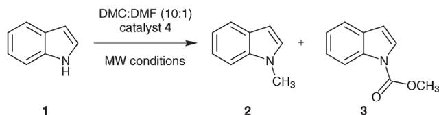
**Fig. 1** Reaction of indole (1) with DMC forming *N*-methylindole (2) and *N*-(methoxycarbonyl)indole (3) catalysed by the basic ionic liquid tributylmethylammonium methylcarbonate (4).
