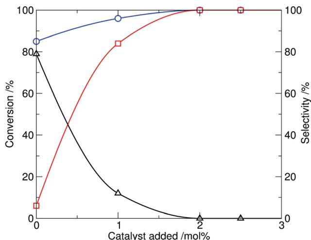
**Fig. 3** Effect of tributylmethylammonium methylcarbonate catalyst loading on the methylation of indole with DMC, showing conversion of indole (**1**, circle) and selectivity to *N*-methylindole (**2**, square) and *N*-(methoxycarbonyl)indole (**3**, triangle) at 230 °C, 20 min reaction time.
