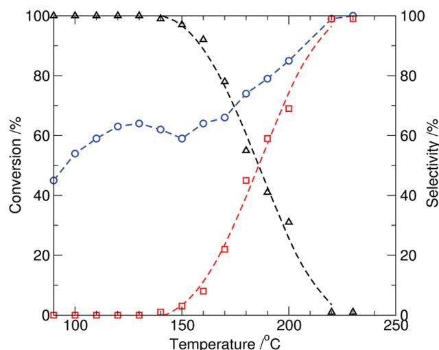
**Fig. 2** Conversion of indole (**1**, circle) and relative selectivity to the two observed products, *N*-methylindole (**2**, square) and *N*-(methoxycarbonyl)indole (**3**, triangle), from the reaction of indole with DMC catalysed by tributylmethylammonium methylcarbonate (10 mol%) as a function of temperature under batch microwave heating (10 min, reaction time).
