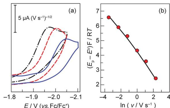
**Fig. 2** (a) Overlay of representative CVs taken of a 0.2 mM solution of **1** in acetonitrile with 0.03 (—•—), 0.3 (—•—), and 3 (—•—)  $\text{V s}^{-1}$  scan rates, using a glassy carbon electrode. (b) Plot of  $(E_p - E^0)F/RT$  vs.  $\ln$  of scan rate ( $E^0 = -2.14$  V, taken from system **2**). Experimental data (●), simulated curve (—) plotted for  $k_s = 0.24$   $\text{cm s}^{-1}$  and  $k_{\text{PT}} = 8.5 \times 10^6$   $\text{s}^{-1}$ .
