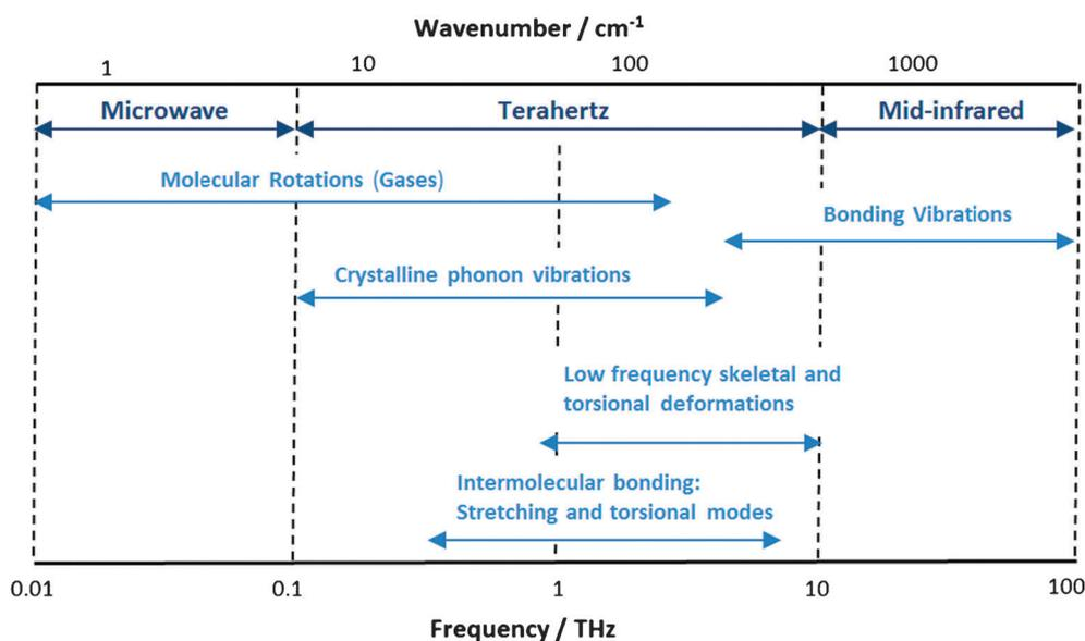
Fig. 1 Molecular modes and activity in the terahertz region of the electromagnetic spectrum.
