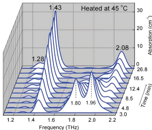
**Fig. 6** THz absorption spectra (with baselines corrected) of D-glucose monohydrate being heated at 45 °C for about 27 min. The numbers mark the positions of absorption peaks. The absorption peaks at 1.80 and 1.96 THz decreased and the absorption peaks at 1.28, 1.43, and 2.08 THz increased over time due to the reduction of D-glucose monohydrate and augment of anhydrous D-glucose during the dehydration. (Reproduced with permission of Elsevier from ref. 47).
