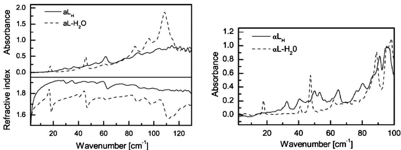
**Fig. 3** Terahertz absorption spectra and frequency dependent refractive indices of  $\alpha$ -lactose anhydrate ( $\alpha$ L<sub>H</sub>) and  $\alpha$ -lactose monohydrate ( $\alpha$ L-H<sub>2</sub>O) at 293 K (left) and 90 K (right). (Reproduced with permission of Elsevier from ref. 14).
