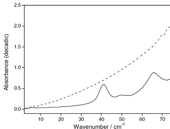
Fig. 2 Absorbance spectra of indomethacin crystalline (solid line) and amorphous (dashed line) 75% in polyethylene. Reproduced with permission of Elsevier from ref. 10.
