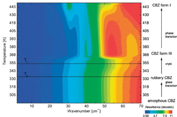
**Fig. 4** Contour plot of the non-isothermal heating of amorphous carbamazepine (CBZ) from room temperature. The sample was heated from 293 K until its melting point at a heating rate of 1 K min<sup>-1</sup>. (Reproduced with permission of John Wiley & Sons, Inc. from ref. 42.)
