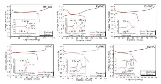
Fig. 3 The charge–discharge curves of Prussian blue analogues KMFe(CN)<sub>6</sub>–Na cells at the third cycle with a current of C/20. Insets show their corresponding chronoamperograms.
