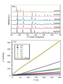
**Fig. 2** (a) XRD patterns of Prussian blue compounds. (b)  $\chi_{\rm m}^{-1}$ -T plot of Prussian blue compounds.
