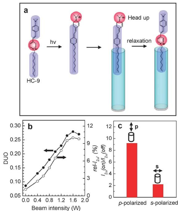
**Fig. 8** A schematic illustration of the shift of the hydrophilic part (red) to the very end of the head part in the photoexcited state, and the subsequent insertion into silicalite-1 channels with the tail part first (a). Plots of the DUO and  $\text{rel-}I_{2\omega}$  (in %) with respect to the laser beam intensity (b) and the effect of the beam polarization direction (p or s) on the  $I_{2\omega}(\text{on})$  to  $I_{2\omega}(\text{off})$  ratio (c). (Adopted from ref. 48.)
