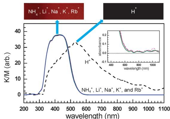
**Fig. 13** Diffuse reflectance spectra of  $[2C^+, (PbS)_{QD}]_Y$  for  $C^+ = NH_4^+, Li^+, Na^+, K^+, Rb^+$ , and  $H^+$  (as indicated) after exposure to the moisture and the corresponding colors (maroon and black for  $C^+$  as indicated). (Adopted from ref. 80.)
