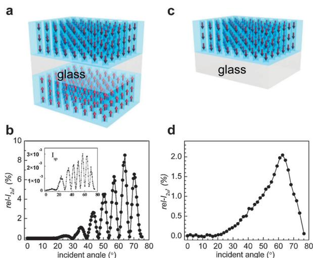
**Fig. 5** A schematic illustration of a glass plate coated with HC-18-incorporating silicalite-1 films on both sides (a) and its typical Maker fringe obtained from the p-polarized laser beam (b). The corresponding Maker fringe obtained from the s-polarized laser beam is shown in the inset. A schematic illustration of a glass plate coated with HC-18-incorporating silicalite-1 film only one side (c) and its typical Maker fringe obtained from the p-polarized laser beam (d). (Adopted from ref. 47.)
