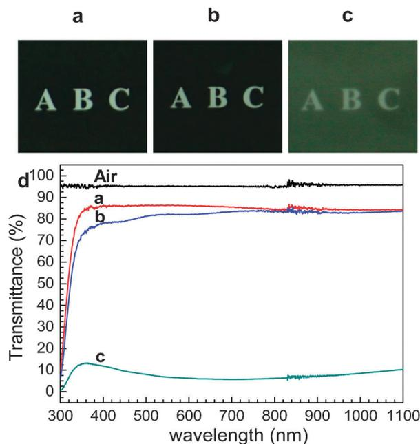
**Fig. 4** Photographs of a 1 mm thick bare glass plate (a), the same glass plate coated with perfect *b*-oriented silicalite-1 films on both sides (b), and the same glass plate coated with randomly oriented silicalite-1 films on both sides (c), and the transmittance spectra of air and three glass plates shown above (as indicated). (Adopted from ref. 50.)
