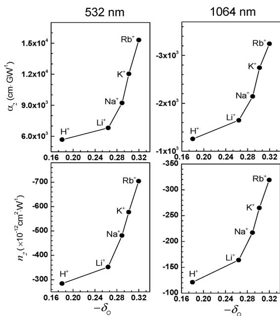
**Fig. 14** Plots of the  $\alpha_2$  (top) and  $n_2$  (bottom) values measured at 532 nm (left) and 1064 nm (right), respectively, with respect to the Sanderson's partial negative charge of oxygen ( $-\delta_O$ ). (Adopted from ref. 80.)
