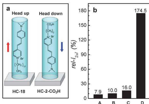
**Fig. 10** A schematic illustration of the orientations of HC-18 and HC-2-COOH in silicalite-1 channels (a) and the comparison of the maximum  $rel-I_{2\omega}$  values obtained from different HC molecules: A: HC-18, B: HC-9\*, C: HC-2-COOH, and D: HC-15. For silicalite-1 films, primarily grown (A–C) and the secondarily grown perfect b-oriented (D).
