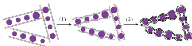
**Fig. 1** Schematic illustration of the synthesis route for silicon nanoparticles inserted into graphene. Grey lines (graphene oxide), black lines (thermally reduced graphene), and purple balls (silicon nanoparticles). (1) Freeze-drying, and (2) thermal reduction.
