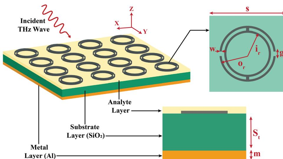
Fig. 1 Schematic diagram of the THz MM sensor-based pesticide detection system, including the unit cell structure and cross-section.
